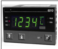
The FUZYPROt 8010 is a 1/8 DIN microprocessor based digital indicator. Available with red or green displays. One latchable relay is fitted as standard, plug-in modules allow two more alarm relays, PV retransmission or transmitter PSU.
