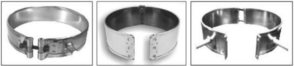
Mica & Mineral Band Heater from Heaters Controls & Sensors are available in various sizes, voltages, wattage's, and constructions to suit every application. The Mica Insulated Band Heater is used for temperatures to 900°F. The Mineral Insulated Band Heaters is used for temperatures to 1400°F. The Mica & Mineral Band Heater can be internally or externally heated, full or split case for easy removal or installation and supplied with various types of leads as shown.
