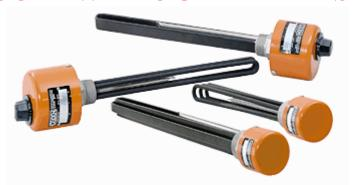
Screw Plug Immersion Heaters are ideal for immersion min liquids, where space and connections are a problem. These Heaters are installed in medium to small size containers at pressures up to 3000 PSI. Watt densities from 90 Watts/sq. inch, Explosion Proof (NEMA 7), Corrosion Resistant (NEMA 4X), and General Purpose Terminal housings are available.
