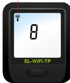
4) RECEIVED SIGNAL STRENGTH INDICATOR (RSSI) (VALUE BETWEEN 0 & 10)
